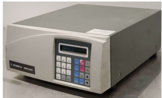
Figure 7. This generator is a fixed 20 kHz frequency and variable 1500 W AC power supply. (Photo courtesy of Sonics & Materials.)
