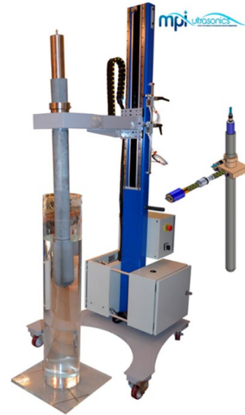
Figure 9. The ultrasonic equipment setup. (Photo courtesy of MPI.)
